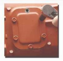
2. Keep aperture plate and bolts in safe place for future use. Clean pad around aperture hole with a gasket scraper. Note: Putting a rag in the aperture hole is recommended to prevent loose gasket material from entering the transmission.
