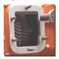
5. Tapped holes in transmission cases require thread/locker compound to keep oil from leaking by the stud or bolt threads.
