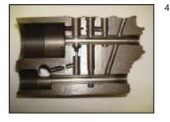
Check the spool bores within the control housing for scoring or excessive wear.
