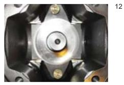
Install the yoke assembly into the cradle bearings, making sure that the long relief on the yoke bearing is located on the pressure side of the pump and the yoke moves freely.
