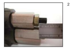
To ensure control is reassembled with the same approximate control settings measure distance from face of adjusting screw plug.
