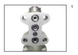
Remove the three sealing o-rings on bottom of control.
