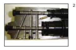
Inspect the springs, spring collar, and spring cup for wear and damage.
