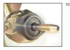
Remove shaft assembly from pump housing.
