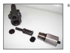
Remove the pressure adjustment screw plug assembly.
