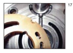
Install the valve plate onto the port plate (lining up the locating pin on the port plate with the alignment slot on the valve plate).
