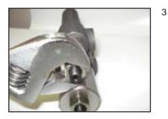
Remove the lock nuts on the pressure adjusting screws.
