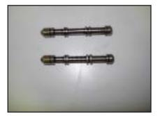
Carefully inspect the spools ensuring the sealing lands are free of any nicks or scratches. Also check the spool ends that contact the spring collar for wear.
